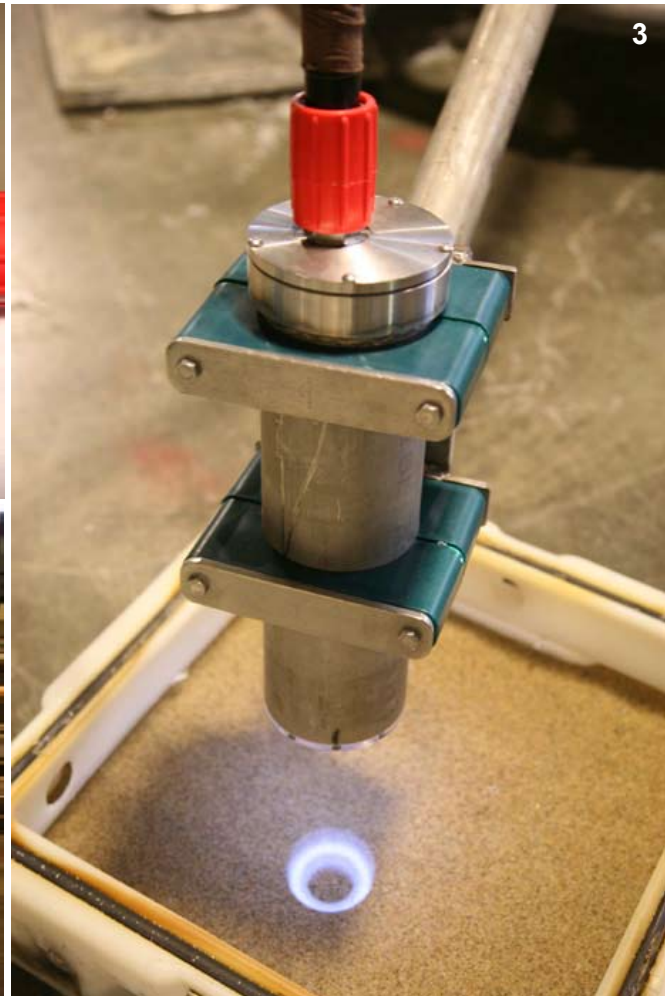
1. GC2450C camera assembly close-up , 2. Platform with sand grain image during initial tests, 3. Camera and light ring during tests
