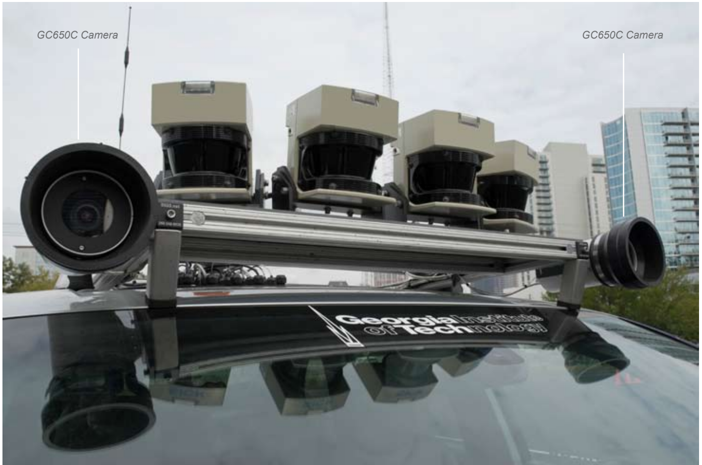
Close-up of the two Prosilica GC650C cameras inside weatherproof housings on either side of the car - Copyright SAIC 2007
