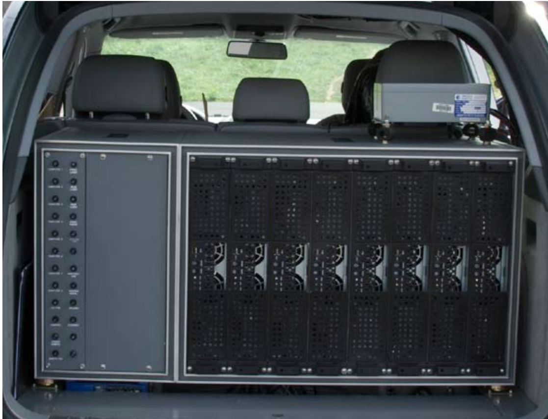
Sting 1's brain - 8 PCs located inside the trunk - Copyright SAIC 2007
