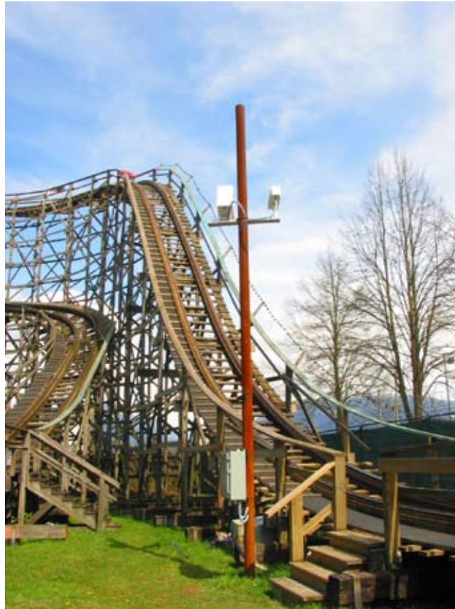
1. Prosilica camera mounted on a mast alongside control box.
