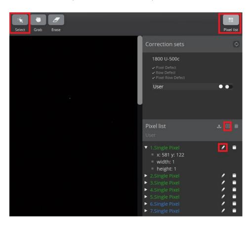
Note that an updated defective pixel list only becomes active after a camera reset. This is Alvium camera firmware behavior.
