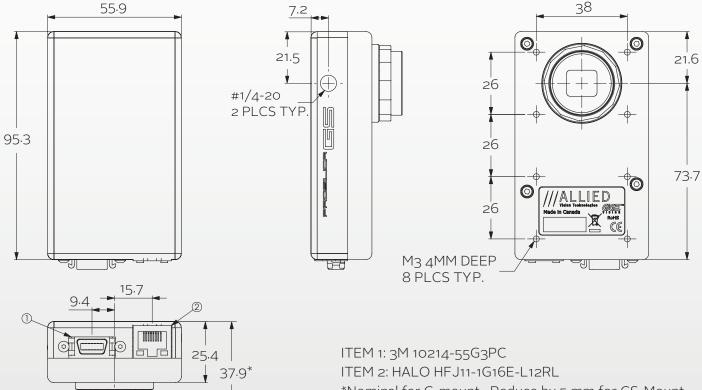
\*Nominal for C-mount. Reduce by 5 mm for CS-Mount. Add 0.3 mm for color option.
