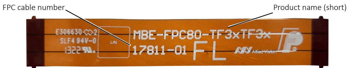
Figure 18: FPC cable number on an Alvium Flex FPC cable
