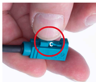
Figure 22: Pressing down the latch (c) of the FAKRA coaxial connector
