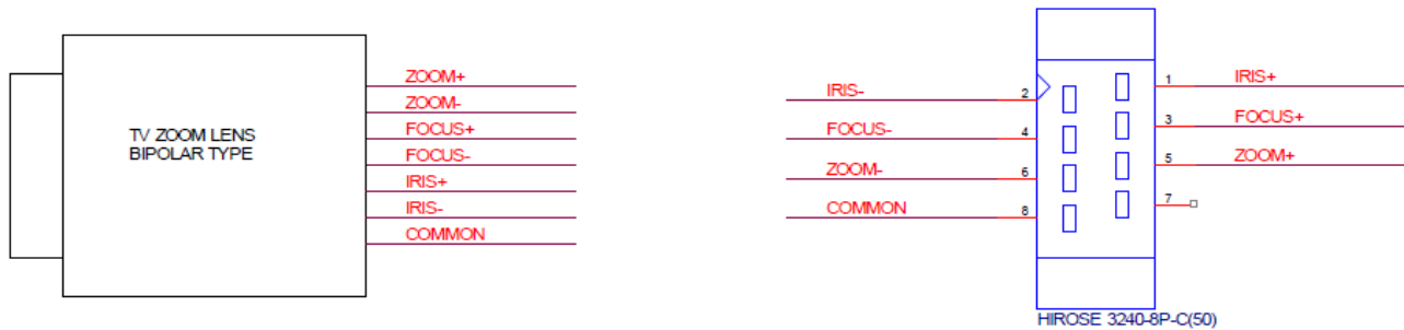
Figure 4 – Direct Drive Lens, bipolar type connection diagram
